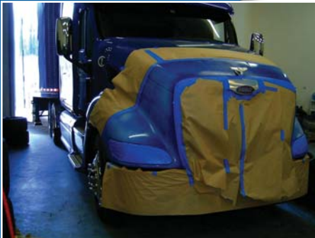
Fresh application of Clear Spray Peel, beginning to cure.
